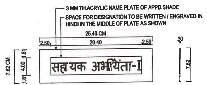
DETAIL OF NAME PLATE 'B' SIDE ELEVATION FOR STAFF CABINS TO BE PASTED AT ENTRANCE
